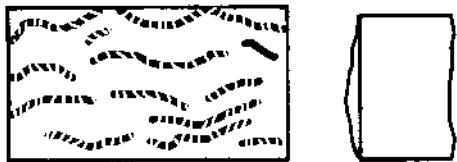
Fig. 7.2 : Hammer Dressed Stone Surface
