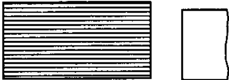
Fig. 7.6 : Closed Picked Stone Surface
